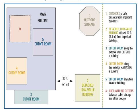
The storage recommendations for idle pallets are shown above. Idle pallets are not of great value. They burn easily and therefore should not be stored near items that are valuable. The heat emitted by a burning pallet will open sprinklers, producing thick smoke and damaging nearby contents.
