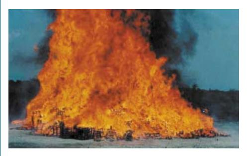
Above are photographs of a fire that was set intentionally to demonstrate the hazard of fire in idle pallets. A total of roughly 2,500 pallets were used. The pile was 12-ft. (4-m) high and 100-ft. (30-m) wide. The second picture shows the fire approximately 15 minutes after ignition. Flames were estimated to be 100-ft. (30-m) high or more.
